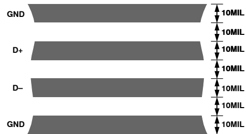
Figure 17. Arrangement of Signal Tracks
